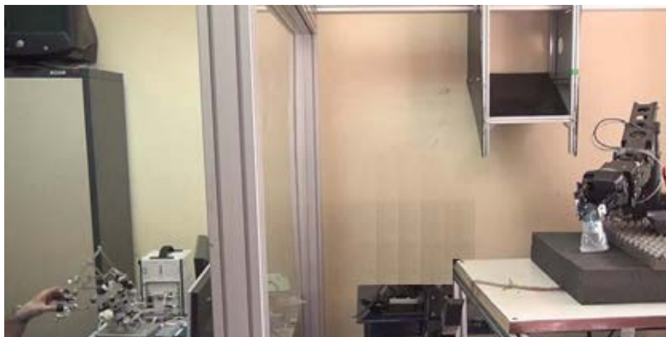
Fig. 3. Operator performing a complex telemanipulation task. These three methods are compared by the execution of the same task: the telemanipulation of a fragile object (a bulb). The steps of the task are:
